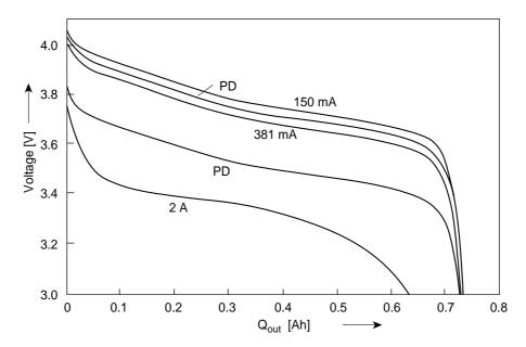
**Figure 6.11:** Measured discharge curves of the CGR17500 Li-ion battery. The top curve is for a DC discharge current of 150 mA. The third curve from the top is for a DC discharge current of 381 mA. The bottom curve is for a DC discharge curve of 2 A. The two remaining curves form the discharge curve including voltage ripple for the current profile shown in Figure 6.10, which has an average value of 381 mA
