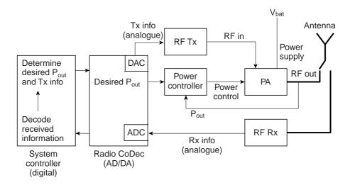
Figure 7.24: PA connections and power control organization in a Spark phone
