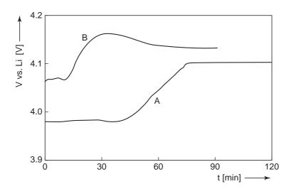
Figure 5.12: Simulated LiCoO<sub>2</sub> electrode potential versus a Li metal reference electrode ([V]) as a function of time (t [min]) for charging regimes A and B; see Table 5.8
