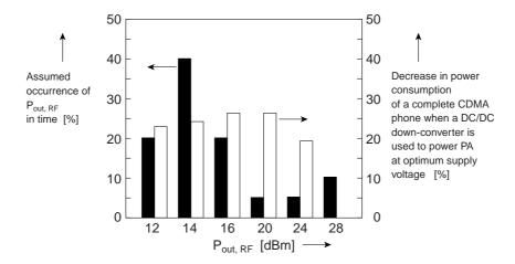
**Figure 7.19:** Reduction in power consumption of a complete CDMA phone at various output power levels  $P_{out,RF}$  (in [dBm]) and the assumed occurrence in time of these output powers (in [%]). Battery voltage  $V_{bal}$ =3.5V
