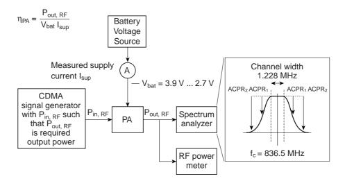
Figure 7.16: Set-up for part 1 of the measurements: no DC/DC converter
