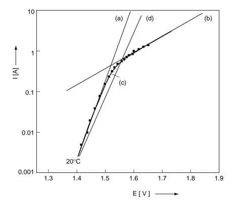
**Figure 4.36:** Same measured Tafel plots (curves (a)-(c)) as shown in Figure 4.35. Also included is the Tafel plot calculated for the evolution of oxygen at the nickel electrode according to (Eq. 4.97) (d) as was included in the NiCd model presented in section 4.2, using optimized parameter values for  $(I_{O_2}^o)_{N_i}^O$  and  $\alpha_{O_2}$ ; see Table 4.4
