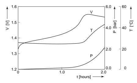
**Figure 4.43:** Simulated battery voltage (V [V]), internal oxygen gas pressure (P [bar]) and temperature (T [ $^{\circ}$ C]) as a function of time (t [hours]) during charging at 25 $^{\circ}$ C ambient temperature at a 1 C rate. The optimized parameter values given in Table 4.4 were used
