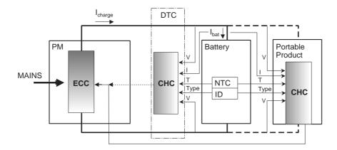
Figure 2.3: Incorporation of the charge monitor and control functions (CHC) inside the portable product
