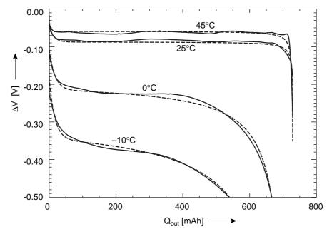
**Figure 6.22:** Experimental differential battery discharge curves obtained for a differential rate of 0.4 C as a function of the charge obtained from the battery  $Q_{out}$  [Ah] at  $-10^{\circ}$ C,  $0^{\circ}$ C,  $25^{\circ}$ C and  $45^{\circ}$ C. The dashed curves show the overpotentials calculated with the aid of (Eq. 6.4) using the parameter values listed in Table 6.3
