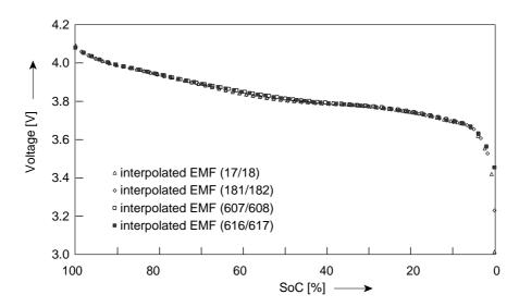
**Figure 6.17:** Measured interpolated EMF curves for different charge/discharge cycles at 25°C. Cycle 17/18 ( $\Delta$ ), cycle 181/182 ( $\diamondsuit$ ), cycle 607/608 ( $\square$ ), cycle 616/617 ( $\blacksquare$ ). The x-axis shows SoC [%], normalized to maximum capacity (see text)
