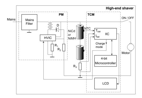
Figure 2.10: Battery Management System inside a high-end shaver
