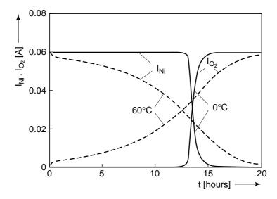
**Figure 4.44:** Simulated partial nickel ( $I_{Ni}$  [A]) and oxygen ( $I_{O_2}$  [A]) currents as a function of time (t [hours]) in the nickel electrode during charging at a rate of 0.1 C at 0 °C and 60°C ambient temperature. The optimized parameter values given in Table 4.4 were used
