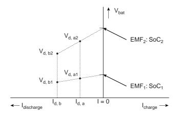
Figure 6.13: Basic concept of linear extrapolation to assess the EMF voltage of a battery
