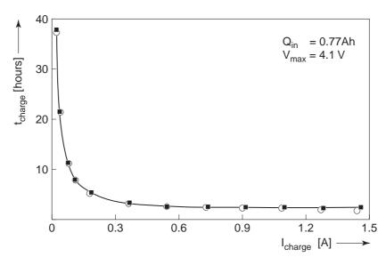
**Figure 4.51:** Simulated (o) and experimental ( $\blacksquare$ ) charge time necessary to charge a Li-ion battery to a capacity of 770 mAh ( $t_{charge}$  [hours]) as a function of the charge current ( $I_{charge}$  [A]) during CC/CV charging with  $V_{max} = 4.1$  V in CV mode at a battery temperature of 25°C
