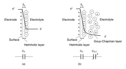
**Figure 3.5:** Helmholtz model (a) and Gouy-Chapman model (b) of the electrical double-layer at an electrode/electrolyte interface. The electrode is assumed to be positively charged and hence to attract negative ions from the electrolyte in this example. The electrode potential is  $\phi^s$  (s=solid) and the bulk electrolyte potential is  $\phi^s$  (l=liquid)
