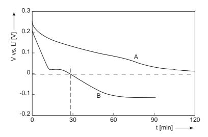
**Figure 5.13:** Simulated  $LiC_6$  electrode potential versus a Li metal reference electrode ([V]) as a function of time (t [min]) for charging regimes A and B. The negative electrode capacity was 850 mAh
