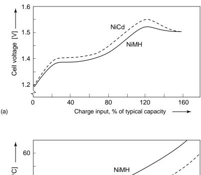
**Figure 5.3:** Comparison of typical characteristics of NiCd (dashed curves) and NiMH batteries (solid curves) during charging at a moderate constant-current charge rate: (a) voltage characteristic (b) corresponding temperature development (measured curves redrawn from [1] with permission)
