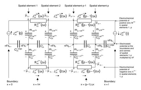
**Figure 4.13:** Simulation model in the chemical domain for one-dimensional mass transport of a charged species in the x-direction in the presence of an electrical field in, for example, the system depicted in Figure 4.12
