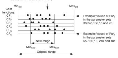
**Figure 4.27:** Simplified schematic representation of the definition of a new range for parameter  $Par_k$ . In the last step shown at the bottom, the values of  $Par_k$  in five parameter sets that yield the five lowest values of cost function  $CF_i$  are shown on each horizontal line
