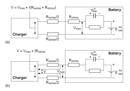
**Figure 5.10:** Two methods for controlling  $V_{max}$  in CV mode: (a) 'resistance-free' measurement by means of current interruption and (b) using additional currentless voltage sense lines. The battery is represented by a simple model
