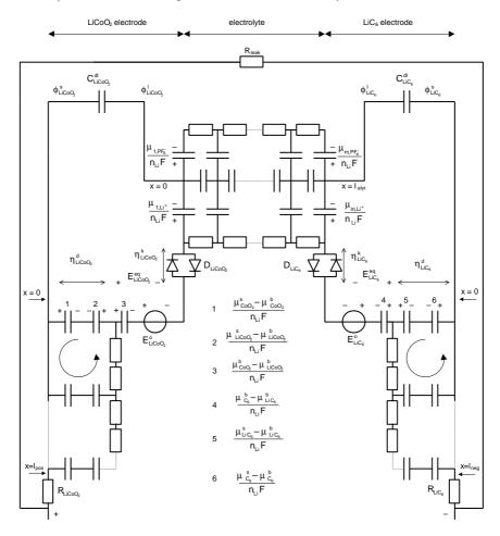
**Figure 4.23:** Alternative simulation model based on that shown in Figure 4.22 with modified definitions of capacitances to allow a distinction to be made between the true equilibrium potential and the diffusion overpotential due to diffusion of Li<sup>+</sup> ions in the electrodes. Moreover, the RC-ladder networks in both electrodes have been rearranged
