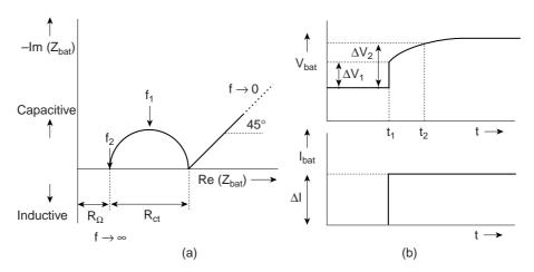
**Figure 6.4:** (a) Measurement of battery impedance in the frequency domain: simplified polar plot showing battery impedance as a function of frequency, (b) Measurement of voltage differences  $\Delta V_I$  and  $\Delta V_2$  after the application of a current step  $\Delta I$  in the time domain
