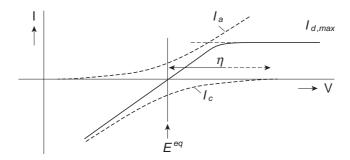
**Figure 3.4:** Current-voltage relationship for an electrode reaction in which the anodic reaction is diffusion-limited at higher anodic reaction currents
