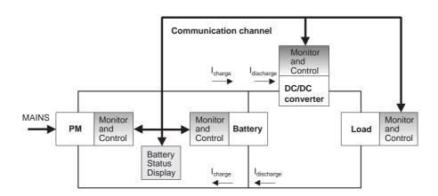
Figure 2.1: A general Battery Management System (BMS)
