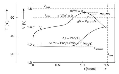
**Figure 5.1:** Overview of end-of-charge triggers based on voltage and temperature measurements. Typical shape of battery voltage (V[V]) and temperature  $(T[^{\circ}C])$  for charging a NiCd battery at a 1 C charge rate at 28°C ambient temperature. These curves have been drawn by hand as an illustration of their typical shape
