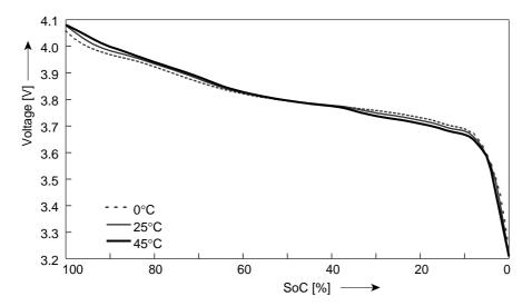
**Figure 6.15:** Measured EMF curves obtained in voltage relaxation after discharge steps at different temperatures:  $0^{\circ}$ C,  $25^{\circ}$ C and  $45^{\circ}$ C. The x-axis shows SoC [%], normalized to maximum capacity (see text)
