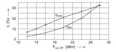
**Figure 7.18:** Efficiency without ( $\eta_{PA}$ , from part 1) and with ( $\eta_{total}$ , from part 2) a DC/DC down-converter at various output powers  $P_{out,RF}$ ,  $V_{bat}$ =3.5V
