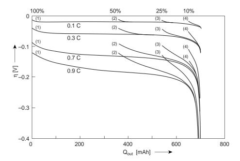
**Figure 6.20:** Simulated overpotentials  $\eta$  [V] versus charge obtained from the battery ( $Q_{out}$  [mAh]) for various discharge rates (0.1 C, 0.3 C, 0.7 C and 0.9 C) for a complete discharge (1), discharge from 50 % SoC (2), discharge from 25% SoC (3) and discharge from 10 % SoC (4) at 25°C. The Li-ion model described in chapter 4 was used in the simulations
