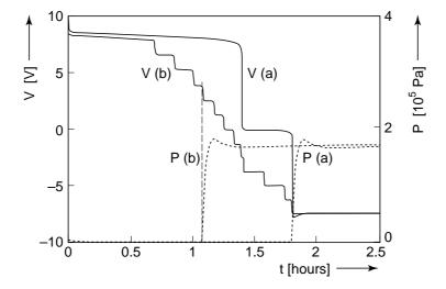
**Figure 4.47:** Simulated voltage (V[V]) and internal oxygen gas pressure  $(P[10^5 Pa])$  as a function of time (t[hours]) of a battery pack with six NiCd cells connected in series during discharging at a 1 C rate and at an ambient temperature of 25°C. Curves (a) represent the situation when all six cells have the same capacity; see Table 4.4. Curves (b) represent the situation when the six cells decrease in steps of 10% of the capacity indicated in Table 4.4
