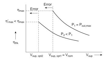
**Figure 7.13:** PA efficiency  $(\eta_{PA})$  versus supply voltage  $(V_{sup})$  for maximum output power  $P_I$  and for  $P_2 < P_I$
