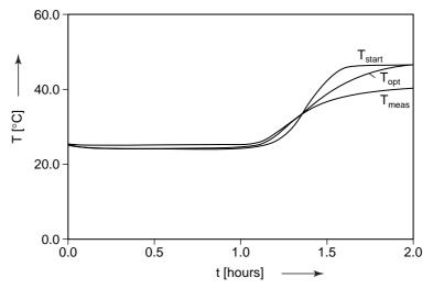
**Figure 4.30:** Simulated  $(T_{start} [^{\circ}C] \text{ and } T_{opt} [^{\circ}C])$  and measured  $(T_{meas} [^{\circ}C])$  battery temperature versus time (t [hours]). See Figure 4.28 for conditions
