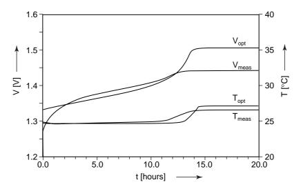
**Figure 4.32:** Simulated ( $V_{opt}$  [V]) and measured ( $V_{meas}$  [V]) battery voltage plotted along the left y-axis and simulated ( $T_{opt}$  [°C]) and measured ( $T_{meas}$  [°C]) battery temperature plotted along the right y-axis versus time (t [hours]). See Figure 4.31 for conditions
