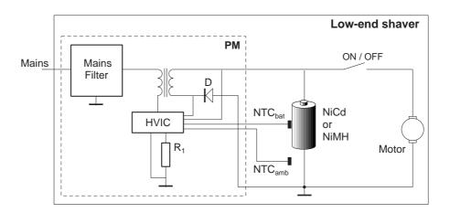
Figure 2.9: Battery Management System inside a low-end shaver
