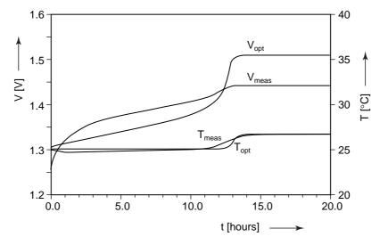
**Figure 4.38:** Simulated ( $V_{opt}$  [V]) and measured ( $V_{meas}$  [V]) battery voltage plotted along the left y-axis and simulated ( $T_{opt}$  [°C]) and measured ( $T_{meas}$  [°C]) battery temperature plotted along the right y-axis versus time (t [hours]). See Figure 4.37 for conditions
