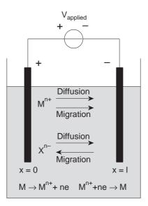
**Figure 4.12:** Schematic representation of an electrochemical cell with two metal (M) electrodes placed in an ideal solution using a  $M^{n+}X^{n-}$  binary salt as the electrolyte, with the  $M^{n+}$  and  $X^{n-}$  ions being transported by combined diffusion and migration
