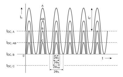
Figure 7.3: Collector currents of different PA classes
