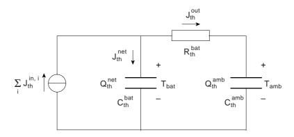
**Figure 4.15:** Simulation model in the thermal domain that describes the temperature development in a battery
