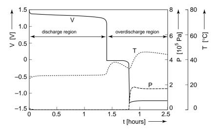
**Figure 4.46:** Simulated battery voltage (V[V]), internal oxygen gas pressure ( $P[10^5 \text{ Pa}]$ ) and battery temperature ( $T[^{\circ}\text{C}]$ ) curves as a function of time (t[hours]) during discharging and overdischarging at an ambient temperature of 25°C at a 1 C discharge rate. The optimized parameter values given in Table 4.4 were used
