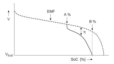
**Figure 6.19:** Schematic representation of EMF (dashed) and discharge (solid) curves leading to zero remaining capacity ( $Cap_{rem}$ =0) at B% SoC
