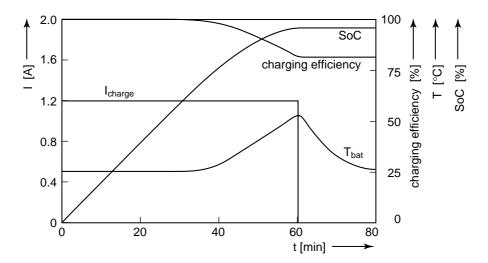
**Figure 5.7:** Simulated charge current ( $I_{charge}$  [A]), State-of-Charge (SoC [%]), charging efficiency [%] and battery temperature ( $T_{bat}$  [°C]) as functions of time (t [min]) for *galvanostatic* charging of a NiCd battery model for one hour using 1.2 A at 25°C ambient temperature. The parameter set of Tables 4.3 and 4.4 was used.
