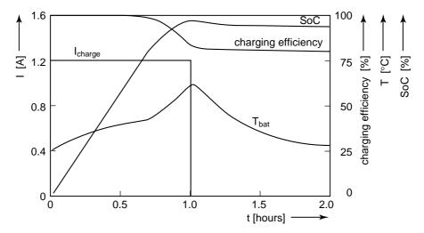
**Figure 5.5:** Simulated charge current ( $I_{charge}$  [A]), State-of-Charge (SoC [%]), charging efficiency [%] and battery temperature ( $T_{bat}$  [°C]) as functions of time (t [hours]) for charging for one hour with a current of 1.2 A at 25°C ambient temperature. A NiCd battery model with the parameter set of Tables 4.3 and 4.4 was used in the simulation model shown in Figure 5.4
