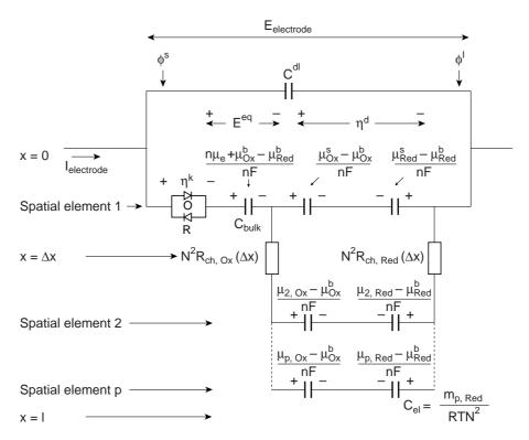
**Figure 4.10:** Adapted simulation model of Figure 4.9 with altered definitions of the capacitances to allow distinction between the true equilibrium potential  $E^{eq}$  and the diffusion overpotential  $\eta^d$ . The model is represented entirely in the electrical domain
