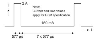
Figure 6.10: Pulse-shaped current used in experiment 2
