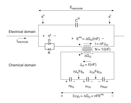
**Figure 4.3:** Simulation model in the electrical and chemical domains for an electrochemical reaction according to (Eq. 4.9). The definition of  $E^{eq}$ , the signs of  $\Delta G$  and  $\eta^k$  and the direction of the current and chemical flow hold for an oxidation reaction (O)
