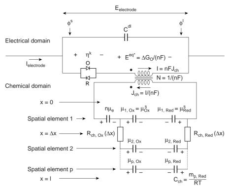
**Figure 4.9:** Simulation model for an electrochemical reaction according to (Eq. 4.9) in the electrical and chemical domains, where mass transport of the Ox and Red species takes place in the electrode in the absence of an electrical field. The definition of  $E^{eq}$ , the signs of  $\Delta G$  and  $\eta^k$  and the directions of the current and chemical flow hold for an oxidation reaction
