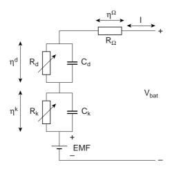
Figure 6.3: Simplified battery model in the electrical domain
