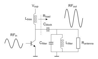
Figure 7.2: Simple representation of a PA [5],[6]
