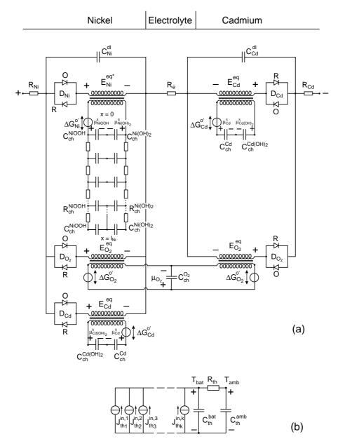
**Figure 4.19:** Simulation model in the electrical, chemical and thermal domains of a rechargeable NiCd battery based on the schematic representation of Figure 4.16. (a) Equivalence of electrochemical behaviour, (b) Equivalence of thermal behaviour
