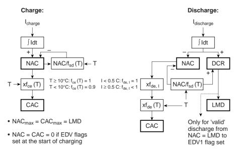
Figure 6.8: Diagram of calculation of remaining capacity in bq2050 (modified from [10])
