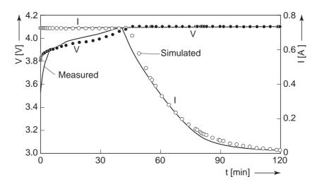
**Figure 4.48:** Simulated (marked lines) and measured (solid lines) voltage (V[V]) and current (I[A]) curves as functions of time (t[min]) for charging a Li-ion battery at a 1 C charge rate in CC mode and a 4.1 V charge voltage in CV mode for two hours in total at a battery temperature of  $25^{\circ}$ C
