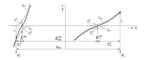
**Figure 3.2:** Current-voltage relation for the positive (+) and negative (-) electrode without mass transport limitations,  $\eta^d$ =0 [6]. The battery voltage  $V_{bal}$ , current I and kinetic overpotentials  $\eta^k_{+/-}$  during charging are shown
