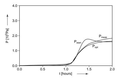
**Figure 4.29:** Simulated ( $P_{start}$  [10<sup>5</sup> Pa] and  $P_{opt}$  [10<sup>5</sup> Pa]) and measured ( $P_{meas}$  [10<sup>5</sup> Pa]) internal oxygen gas pressure versus time (t [hours]). See Figure 4.28 for conditions
