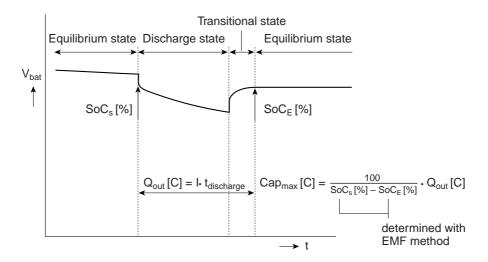
**Figure 6.25:** Simple method for updating  $Cap_{max}$  to take capacity loss into account
