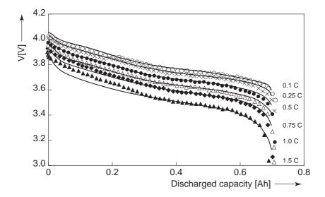
**Figure 4.52:** Simulated (marked lines) and experimental (solid lines) battery voltage curves (V[V]) as functions of the discharged capacity [Ah] during discharging a Li-ion battery with various discharge currents at a battery temperature of 25°C. The discharge rate increases from top to bottom: (o) 0.1 C ( $\times$ ) 0.25 C ( $\bullet$ ) 0.5 C ( $\Delta$ ) 0.75 C ( $\bullet$ ) 1 C ( $\Delta$ ) 1.5 C
