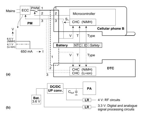
**Figure 2.12:** BMS of a type B cellular phone with a standard Li-ion battery pack and optional NiMH battery pack (a) Control of the charging process (b) Power supply scheme for the various system parts
