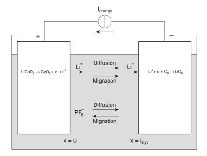
**Figure 4.20:** Schematic representation of the charging of a Li-ion battery, in which Li<sup>+</sup> and PF<sub>6</sub> ions are transported through the electrolyte by means of combined diffusion and migration
