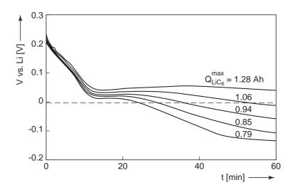
**Figure 5.14:** Simulated LiC<sub>6</sub> electrode potential versus a Li metal reference electrode ([V]) as a function of time for charging regime B and different negative electrode capacities  $Q^{max}_{LiC_6}$
