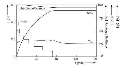
**Figure 5.8:** Same simulated curves as in Figure 5.7 for *thermostatic* charging according to Table 5.3 at 25°C ambient temperature
