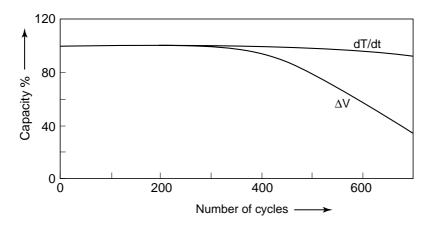
**Figure 5.2:** Battery capacity as a function of the number of charge/discharge cycles of a NiMH battery using either a  $-\Delta V$  or a  $\Delta T/\Delta t$  end-of-charge trigger to terminate fast charging at a 1 C charge rate (measured curves redrawn from [1] with permission)
