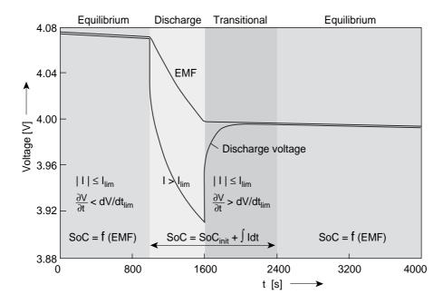
**Figure 6.24:** Simulated EMF (top curve [V]), discharge voltage (bottom curve [V]) and transitions between states as a function of time [s] in the proposed SoC indication system. The battery model shown in Figure 6.3 was used in the simulations, with the overpotential description according to (Eq. 6.4) and an EMF curve derived from measurements
