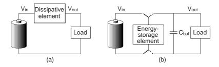
**Figure 7.5:** Two approaches to convert a battery voltage into another voltage. (a): Time-continuous with dissipative element  $(V_{in} > V_{out} \text{ only})$  (b) Time-discrete with energy-storage element
