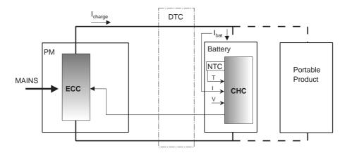
Figure 2.4: Incorporation of the charge monitor and control functions (CHC) inside the battery pack
