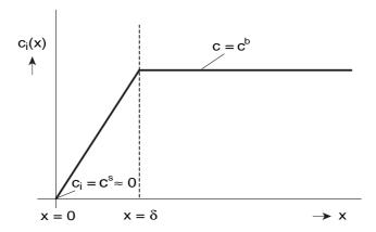
**Figure 3.3:** Concentration  $c_i(x)$  of a diffusing species *i* during stationary diffusion in the *x* direction
