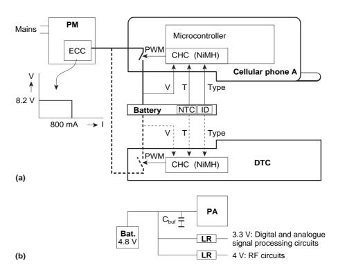
**Figure 2.11:** BMS of a type A cellular phone with a NiMH battery pack: (a) Control of the charging process (b) Power supply scheme for the various system parts
