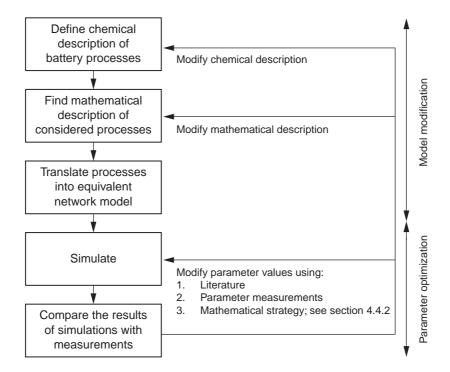
**Figure 4.24:** Set-up of the modelling strategy and iterative process of parameter optimization and model modification aimed at improving the quantitative agreement between the results of simulations and measurements
