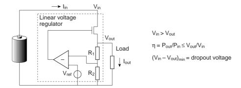
Figure 7.6: Basic schematic representation of a linear voltage regulator
