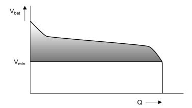
**Figure 2.7:** Schematic representation of a typical battery discharge curve denoting energy loss (shaded area) when the battery voltage is higher than the minimum supply voltage  $V_{min}$  of the load
