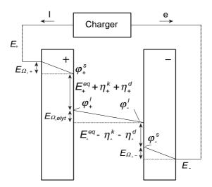
Figure 3.6: Potential development inside a battery during charging; see (Eq. 3.20)
