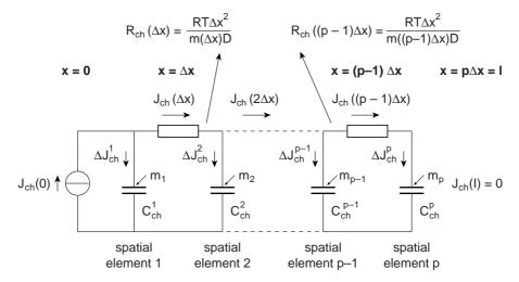
**Figure 4.8:** Simulation model in the chemical domain describing one-dimensional mass transport of a species in the x-direction in the absence of an electrical field
