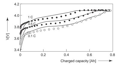
**Figure 4.49:** Simulated (marked lines) and experimental (solid lines) battery voltage (V[V]) curves as functions of the charged capacity [Ah] for charging a Li-ion battery with various charge currents in the CC mode and a 4.1 V charging voltage in the CV mode at a battery temperature of 25°C. The charge rate increases from bottom to top: ( $\circ$ ) 0.1 C, ( $\bullet$ ) 0.5 C, ( $\bullet$ ) 1 C
