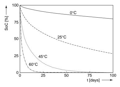
**Figure 4.45:** Simulated SoC as a function of time (*t* [days]) at different ambient temperatures. The optimized parameter values given in Table 4.4 were used
