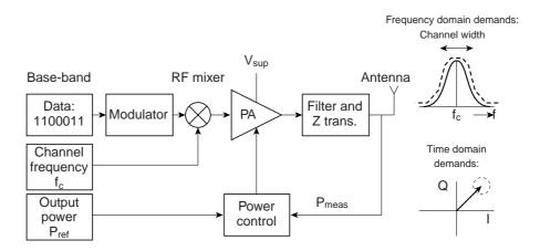
Figure 7.1: Simplified transmit path in a cellular phone from base-band to antenna
